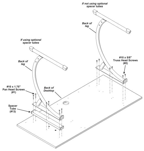
Example only. If optional spacer tubes are used, they must be attached to both legs.
