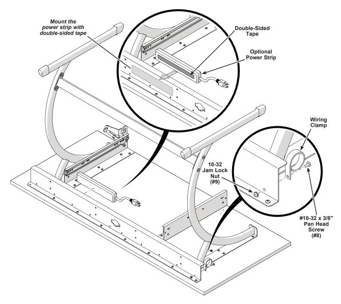
8. Attach wiring clamps (#12) as needed to the stiffener with one #10-32 x 3/8" pan head screw (#8) and 10-32 jam lock nut (#9) in each.
